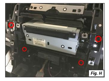
10. Detach the climate control panel and hazard switch bar from the assembly and set aside for reinstallation into the vehicle following dashboard modiciation.
