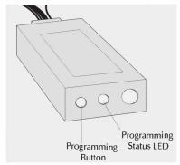
**6.** Hold the IR Transmitter approx. 30cm away from the aftermarket radio and check that each steering wheel button functions correctly.
