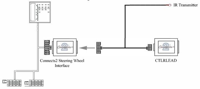
2. Connect the steering wheel interface to the vehicle and the aftermarket head unit using the manual supplied with the steering wheel interface
