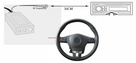
7. Install the IR transmitter where it can point at the radio without any obstructions. The aftermarket head unit needs to be in view of the IR Transmitter in order to receive the steering wheel commands.
