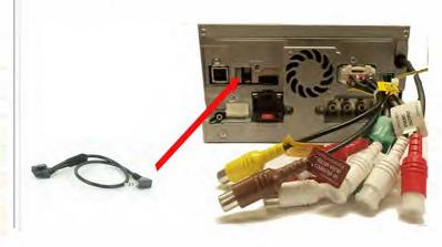
4 Connect the Rear View Camera input to the interface as indicated (Optional if reverse camera fitted).
