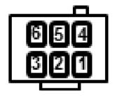
Pin 2: Video-signal rear-view camera Pin 5: Video-signal ground rear-view camera
